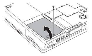
Figure 8-16 Removing the HDD pack cover
